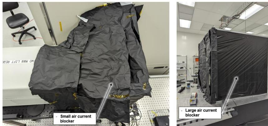
Figure 2-4: Small and large air current blockers used during data collection
